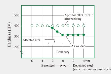
Welding conditions Welding method: TIG welding (argon shield) Preheating: 300 to 400°C Current: 150 to 170A Welding rod: Same material as base steel
