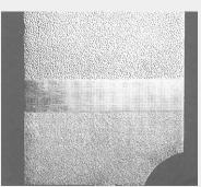
Aged after welded (air cooled at 500°C x 5 Hr)
